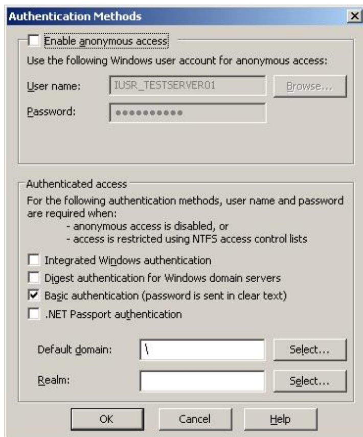
Figure 2: Authentication Method Settings in IIS Manager when FBA is enabled
